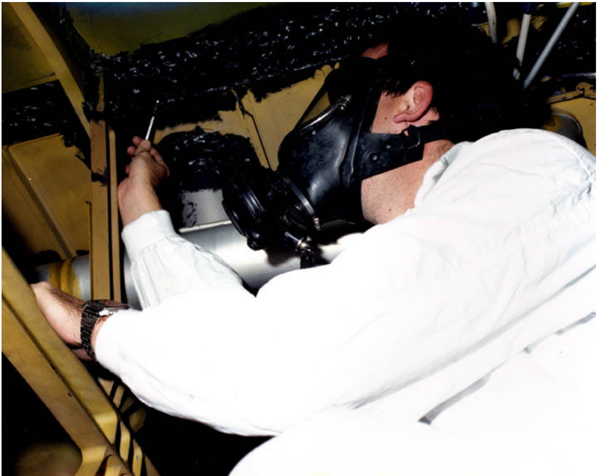
A RAAF maintenance worker finishing the first stage of resealing an F111 fuselage tank. (Stage 2 being another application of sealant.)
