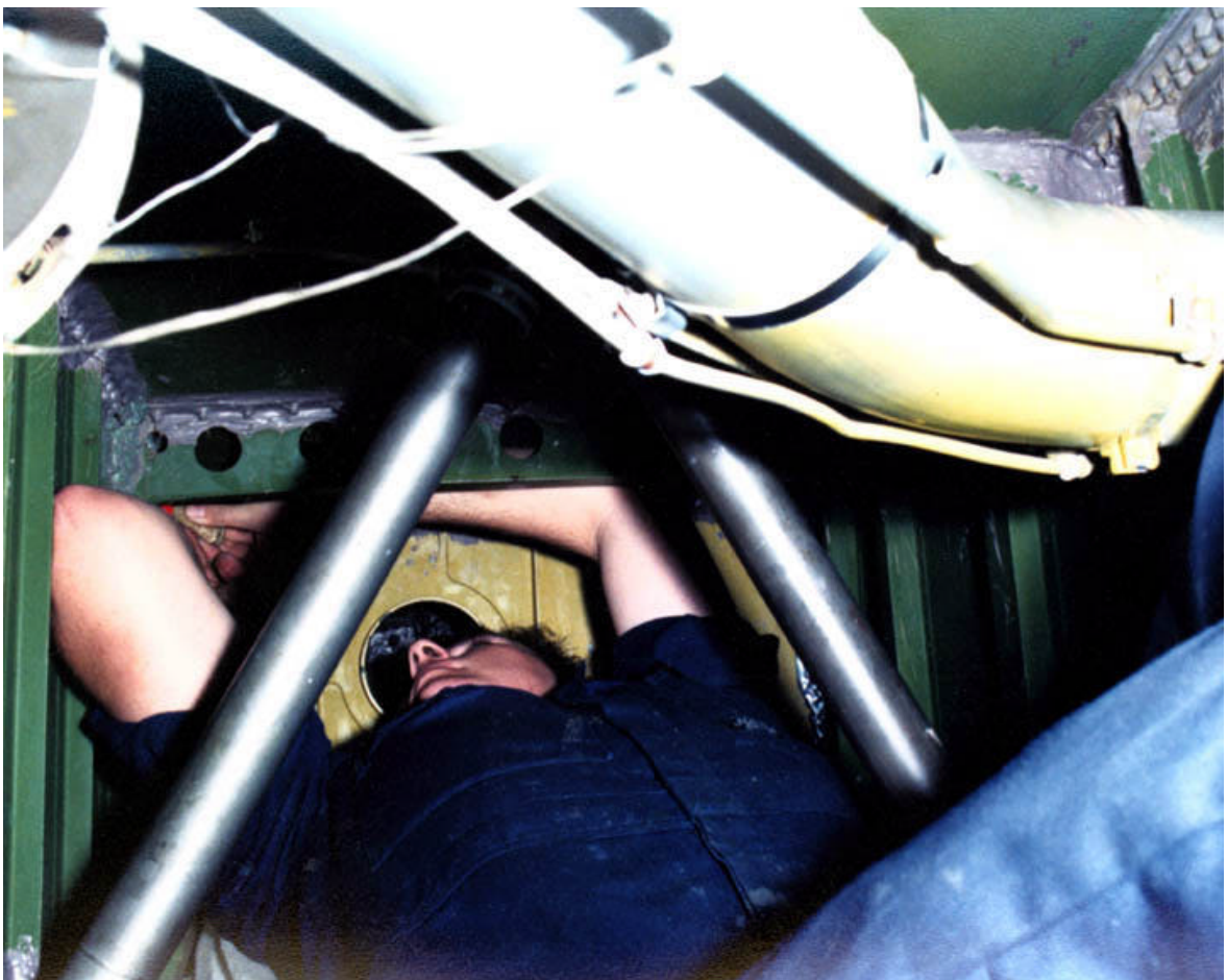
RAAF maintenance worker checking the sealant of a particularly difficult corner in an F111 fuselage tank.
