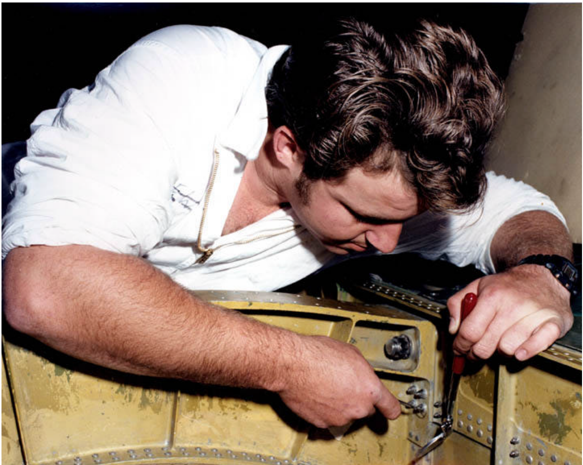
Maintenance worker completing removal of sealant from F111 fuselage tank (using dental pick and mirror) before final clean and application of new sealant
