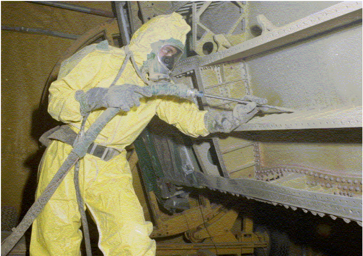
RAAF maintenance worker blasting the interior of an F111 wing fuel tank with walnut shell grit to remove residual sealant in preparation to resealing.
