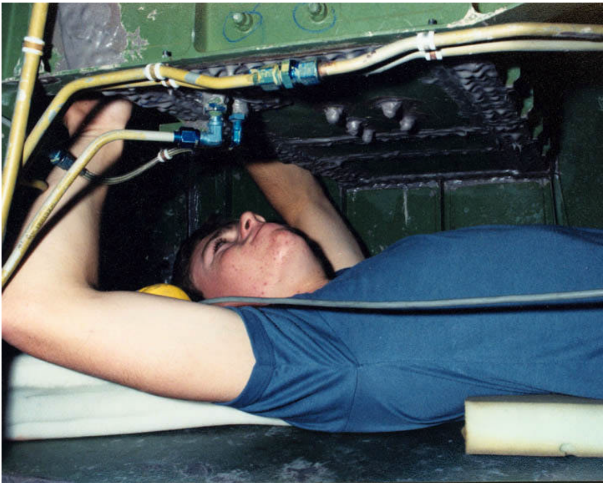
RAAF maintenance worker completes final check to finished sealant application. Note the two bolts at the top of the photo which are yet to be sealed.
