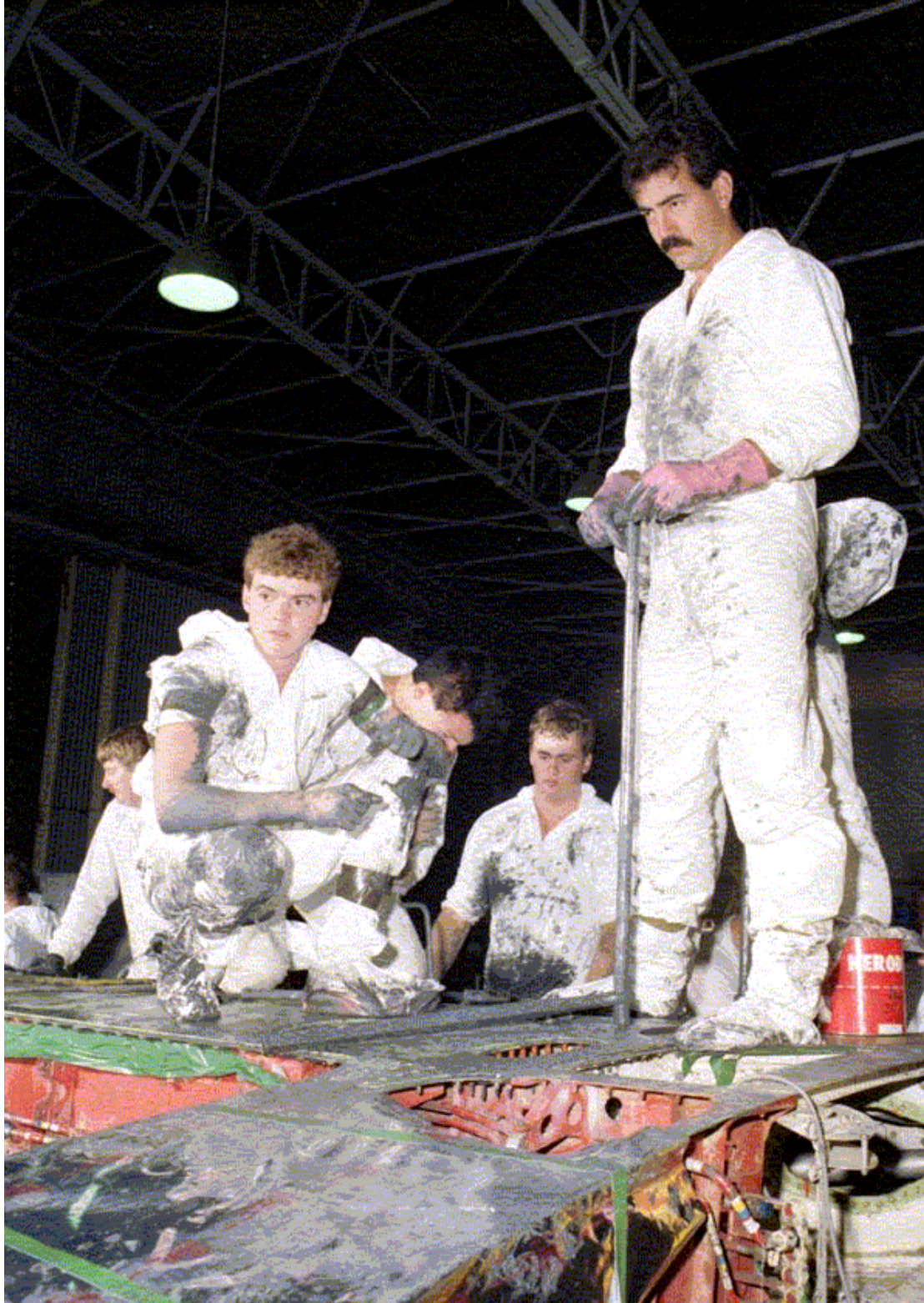
RAAF maintenance workers at the completion of a wing Deseal/Reseal.
