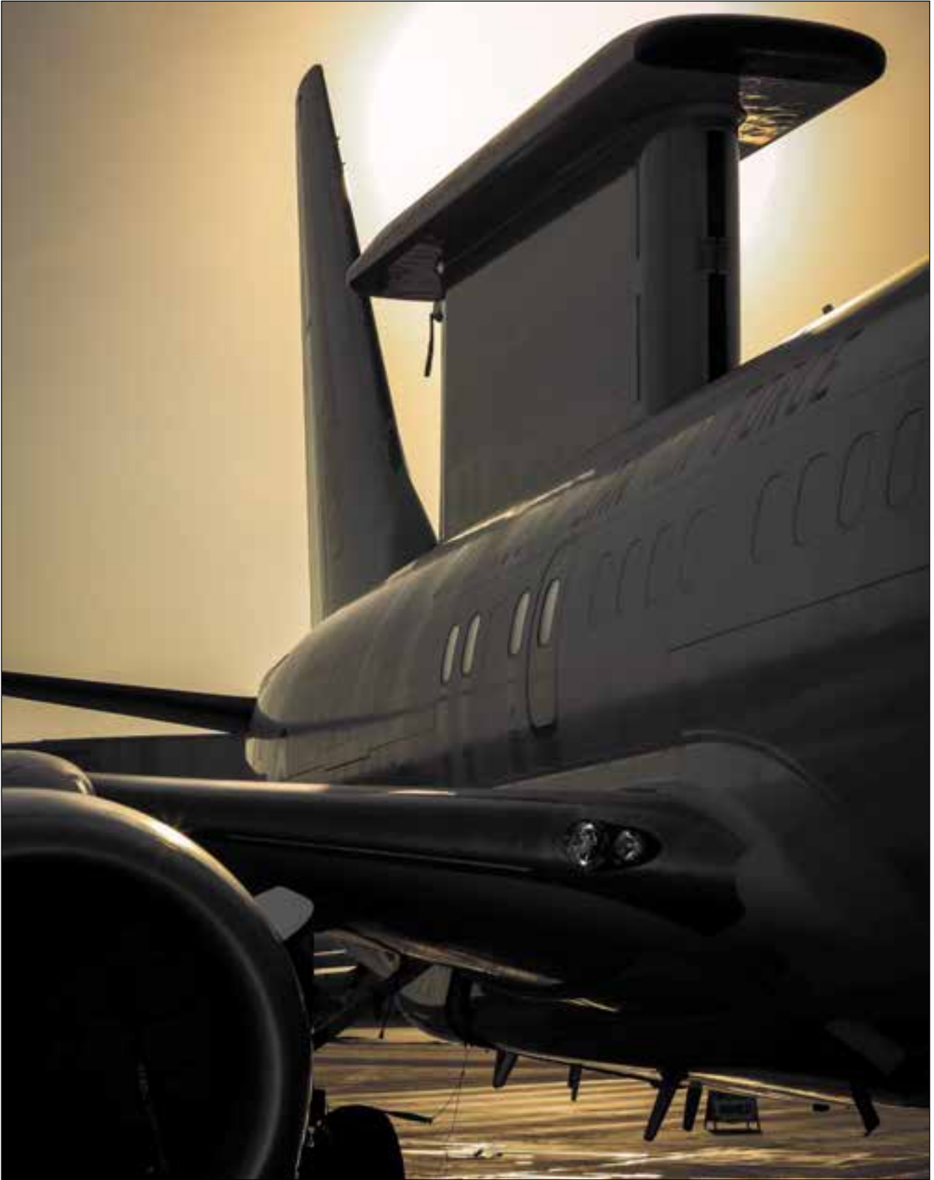
The distinctive addition of an advanced Multi-Role Electronically Scanned Array radar on the RAAF's Boeing E-7A Wedgetail is clearly evident in this image of an aircraft silhouetted by the setting sun in the Middle East, November 2017. Source: Department of Defence
