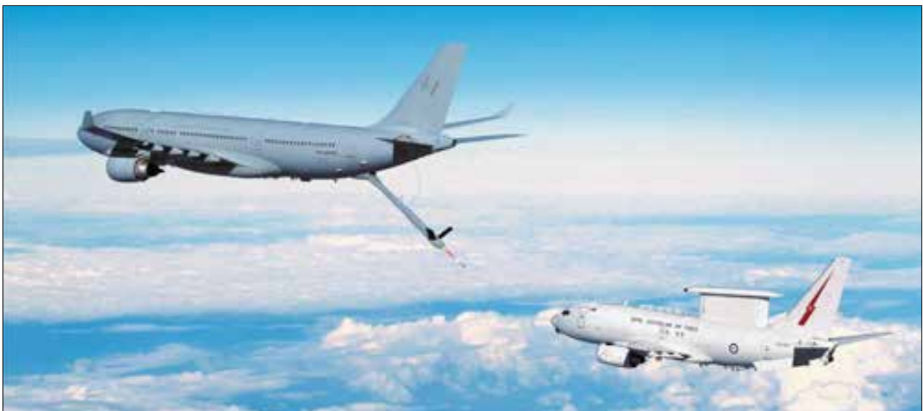
Boeing E-7A Wedgetail A30-001 of No 2 Squadron conducting trials of air-to-air refuelling with Airbus KC-30A A39-005 of No 33 Squadron in the airspace near RAAF Williamtown, New South Wales, in June 2015. Source: Department of Defence
