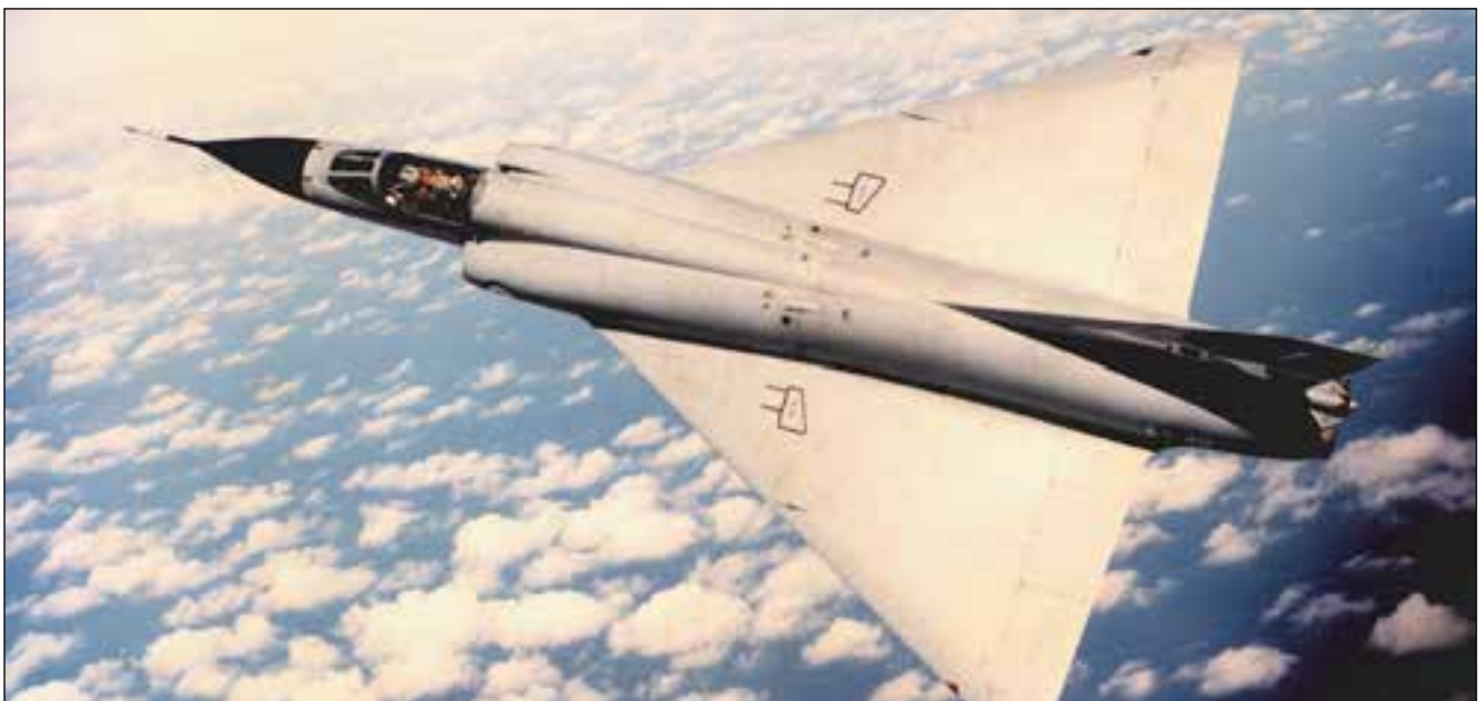
Dassault Mirage IIIO A3-33 showing the sleek lines and the delta wing form that are characteristic of the Mirage family of aircraft. Source: RAAF
